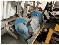
Abrasive wheel guarding and tool rest in place
