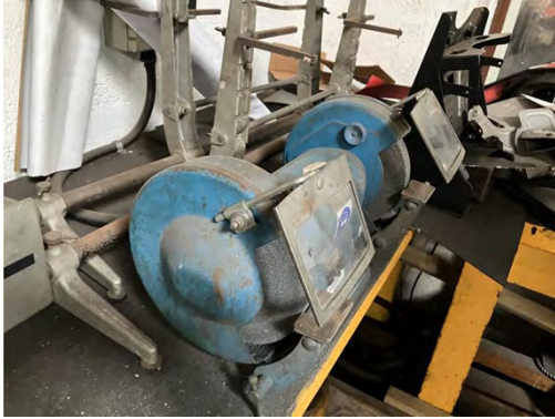
Abrasive wheel guarding and tool rest in place
